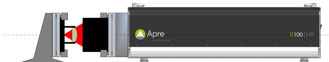
Figure 2: Basic Setup for measuring a convex sphere
