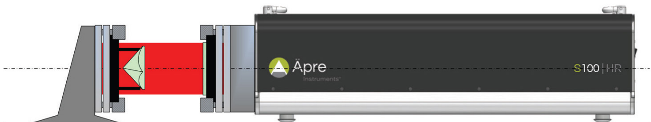
Figure 1: Set up to align the TF using a corner cube retro reflector
