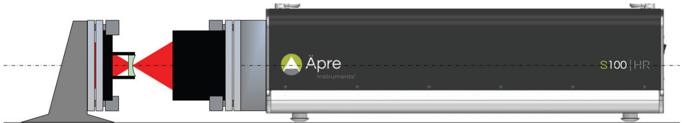
Figure 2: Set up to fine align the TS using the cats eye position
