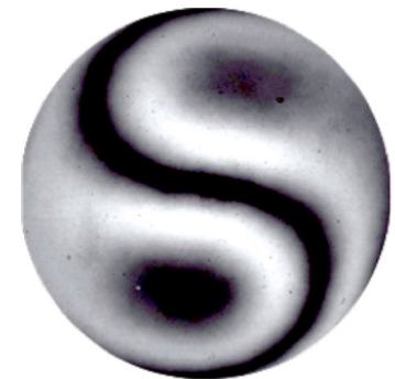
Figure 3: Cat's eye interferogram
