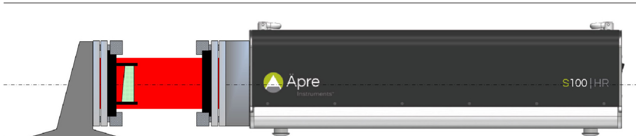
Figure 1: Basic setup for measuring a flat
